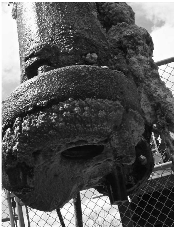
Above: Fats, Oils and Grease buildup on WCCD equipment can require more frequent maintenance and costly repairs.
